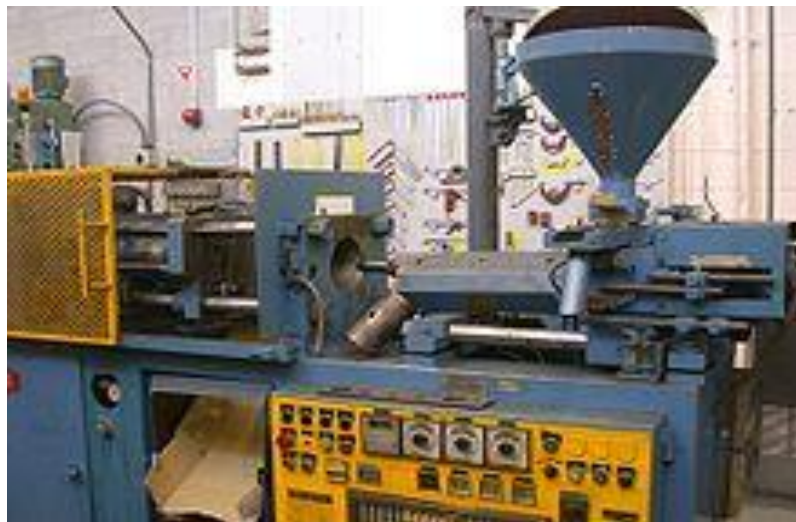
Fig:-2 Hopper, nozzle and die area shown in Small injection molder
